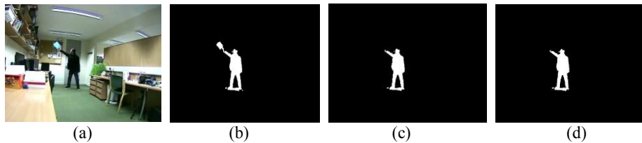
Fig. 4. The experiment of “Raising a book”; (a) source images, (b) foreground detected by GMM, (c) extracted silhouette after using T1FLS, (d) extracted silhouette after using IT2FLS.
